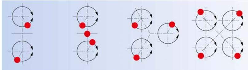
*Picture 3: Hole pattern for adjustable heads with 2, 3 or 4 spindels*
