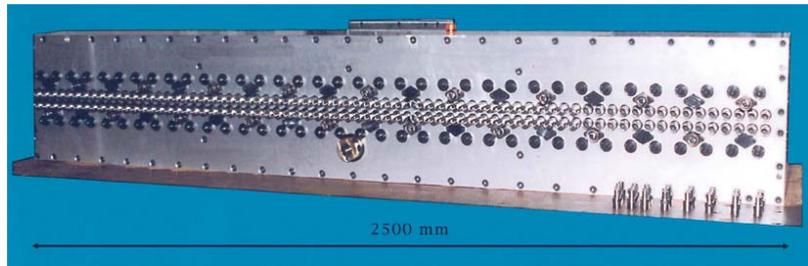
*Picture 4: POLYdrill-Multiple spindle head with 144 spindles at fixed spacings*
