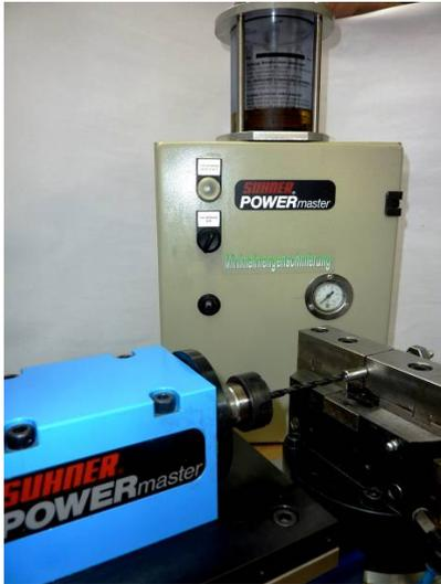
*Drilling of an 8 mm diameter hole in stainless steel 25mm deep using a carbide tool with coolant-through capability, an AccuLube-Booster and a BEX 15 machining unit*
