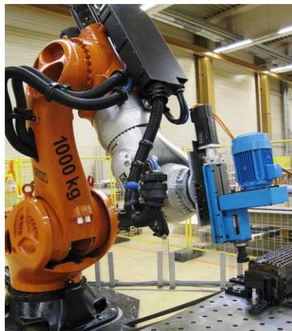
Up to 400Nm torque at the spindle allows for some serious drilling and milling operations. This also demands a „strong“ robot as illustrated in the picture. Clamped-work pieces of alloy steel can be milled completely and followed by a drilling operation of Ø21mm diameter.
