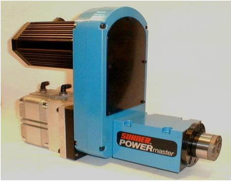
This model includes a specially-designed clamping system. Tool clamping is achieved with ER collets size ER16 or ER25. Collet (Pos. 11) is inside a pressure ring (Pos. 12.) Clamping occurs as the disc-spring-loaded drawbar (Pos. 4) pushes the pressure ring into the spanner ring (Pos. 10). An inline, short-stroke cylinder (Pos. 2) opens the clamp. This type clamping system transmits up to 12Nm of torque.
