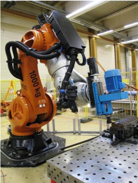
More and more often, machining units are used with strong arm robots in drilling, milling, deburring, grinding or brushing operations.
