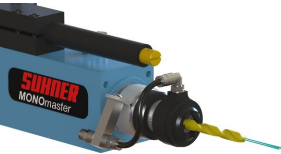
Picture 1: Suhner quill feed unit with coolant through attachment
