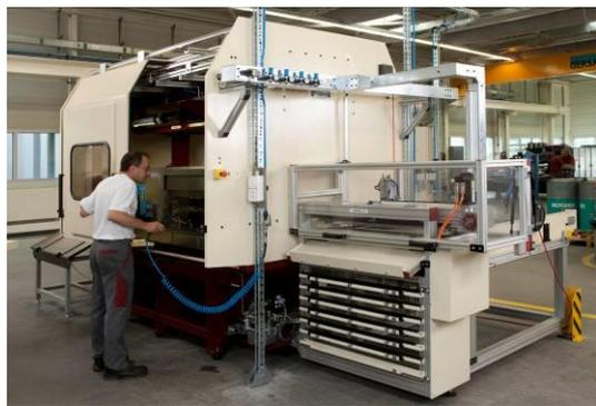
The modular system of *SUHNER* enables the creation of special machines for various applications of profile machining. The illustrated machine produces precision rail guides and was designed and built by the *SUHNER* division for special machines.
