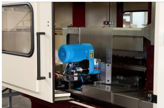
The automatic loading and unloading allows predictable autonomy. Stacks and checking the position and the feeding of bulky workpieces must be adapted individually to the workpieces.
