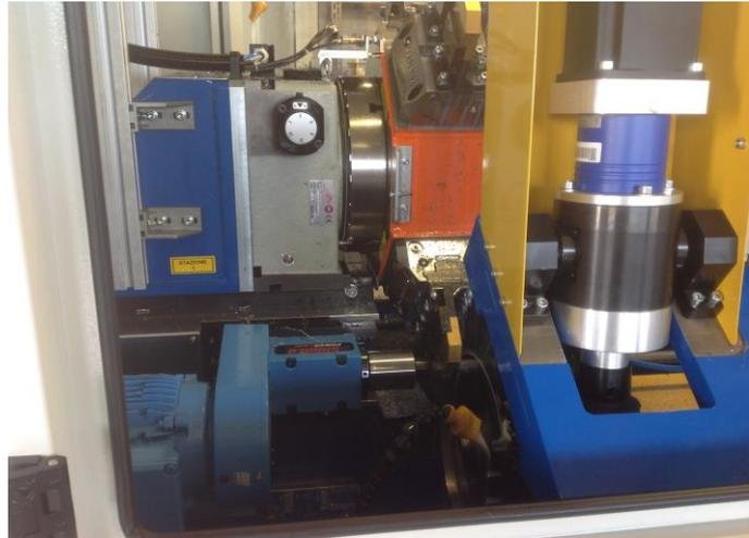
*OD and ID turning station with BEX15-Weldon, 1.5kW motor drive and high precision angular contact spindle bearings*
