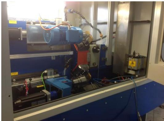
A wealth of experience with operations on transfer machines allows SUHNER to optimize a manufacturing process with standard or custom made solutions for each and every different application. One specific application is for large & long OD threads. These operations are extremely difficult and challenging for manufacturers when trying to obtain short cycle times, simply because an OD threading operation by itself will dictate the overall machine cycle time.
