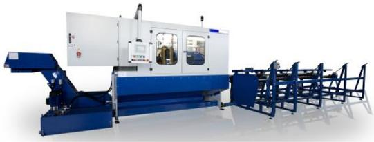
The work piece is fed from bar stock material. After a cut to length operation, it is machined by (3) BEX15 machining units with special Weldon tool holders. Operations include OD & ID and face turning. All units are equipped with a 1.5kW motor and high precision angular contact spindle bearings.
