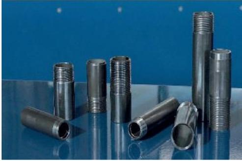
Depending on length, a typical OD thread rolling cycle time ranges between 6 to 10 seconds. Illustrated work pieces are steel tubings as used in the heating product industry. There are 7 part variations, each with a different thread size, pitch and length requirement. Thanks to the application of CNC servo driven spindle and slide components, customers can achieve very short change over time.
